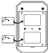
**OPTION 2:** Use the 2 screws and anchors -included- to mount the sliding bracket to the wall as shown in the diagram in desired location (Fig. 3).
